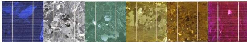
Fig. 3.B.35. multicrystalline silicon wafers; first the blue antireflective standard colour with the best efficiency, the second is the original wafer without reflective layer, then cells with other colours that have different anti-reflective layers, © Sunways
